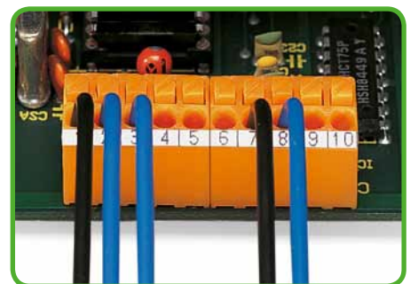
Pin center spacing can be maintained in an assembly.
