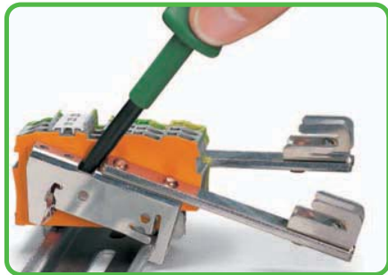
Remove the busbar carrier using an operating tool, type 3, blade (5.5 x 0.8) mm.
