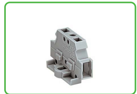
Terminal block with fixing flange, for screw or similar mounting types, fixing hole 3.2 mm Ø (with 209-123 mounting adapter also for DIN 35 rail) Lateral marking facility for miniature WSB Quick marking system, test slot.
