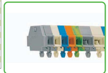
Terminal strip with snap-in mounting feet, for plate thickness 0.6 mm - 1.2 mm (0.02 in - 0.047 in), fixing hole 3.5 mm Ø (fits 210-154 aluminum rail or with 209-120 mounting adapter for DIN 35 rail)
