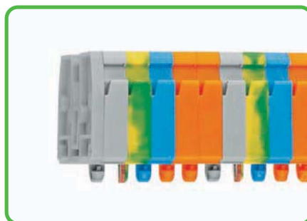
Terminal strips with snap-in mounting feet, for plate thickness 0.6 - 1.2 mm (0.02 - 0.047 in), fixing hole 3.5 +0.1mm Ø
