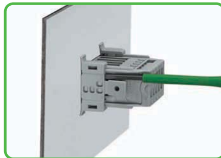
For removal, insert operating tool (blade width 2.5 mm) into release slot.
