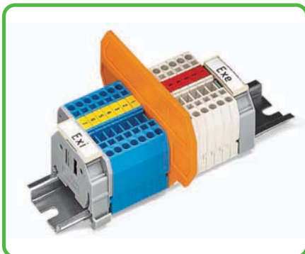
Separator for Ex e/Ex i applications According to EN 50020, a minimum distance of 50 mm must be kept between live parts of Ex e and Ex i circuits. The use of Ex e/Ex i separators is a space-saving solution when Ex e and Ex i terminal blocks are mounted on a common carrier rail. Suitable for 279 to 282 Series terminal blocks. 209-190 for 2-conductor terminal blocks. 209-191 for 2-, 3-, 4-conductor terminal blocks.
