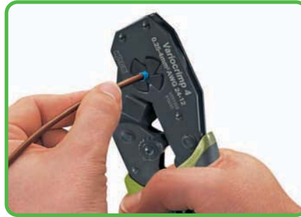
Squeeze handles until ratchet mechanism is released.
