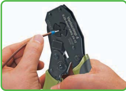
Insert ferruled conductor into crimping station.
